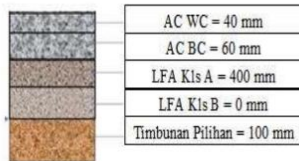
Gambar 2: Detail Perkerasan Metode Bina Marga 2017
