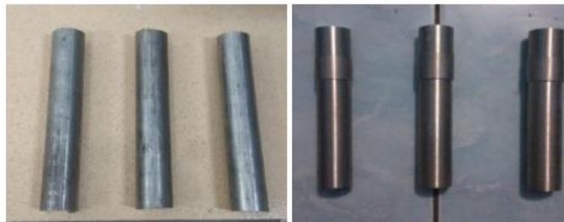
Gambar 1. Stainless steel type 304 (a) Sebelum, (b) Sesudah
