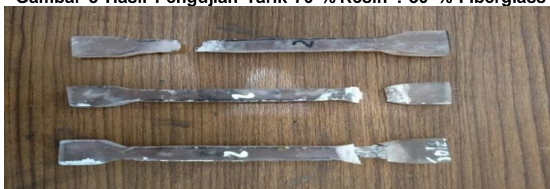
Gambar 4 Hasil Pengujian Tarik 50 % Resin : 50% Fiberglass
