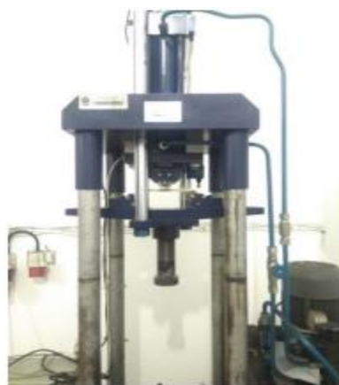
Gambar 2 Alat Uji Three Point Bending
